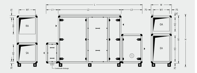
**Important!** Where a system is operated in parallel, the supply air and return air ducts of the two units have to be brought together.
