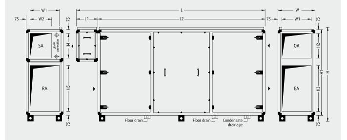
Unit feet 100mm Optionally: adjustable feet from 100 to 120 mm
